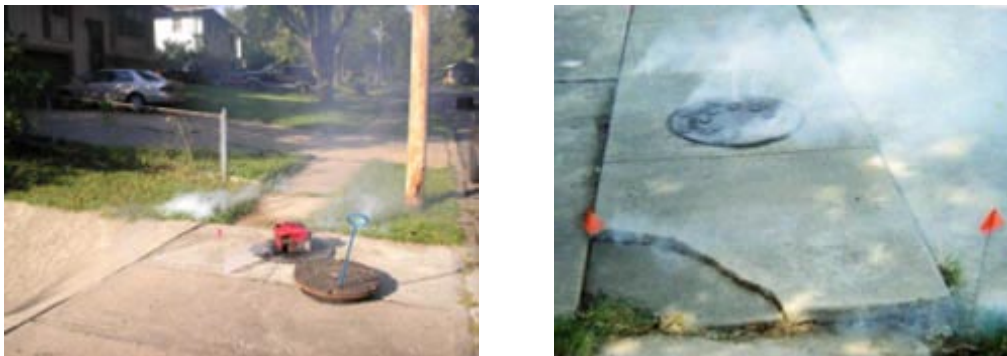
High-capacity blowers are used to pump smoke into a manhole (left photo). In the right photo, smoke is pushed into the system and emerges from cracks in the sidewalk and at a downstream manhole.
